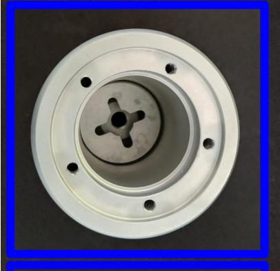
Remove M6x12 caphead screw with 5mm allen key and seperate two halfs of shifter.
